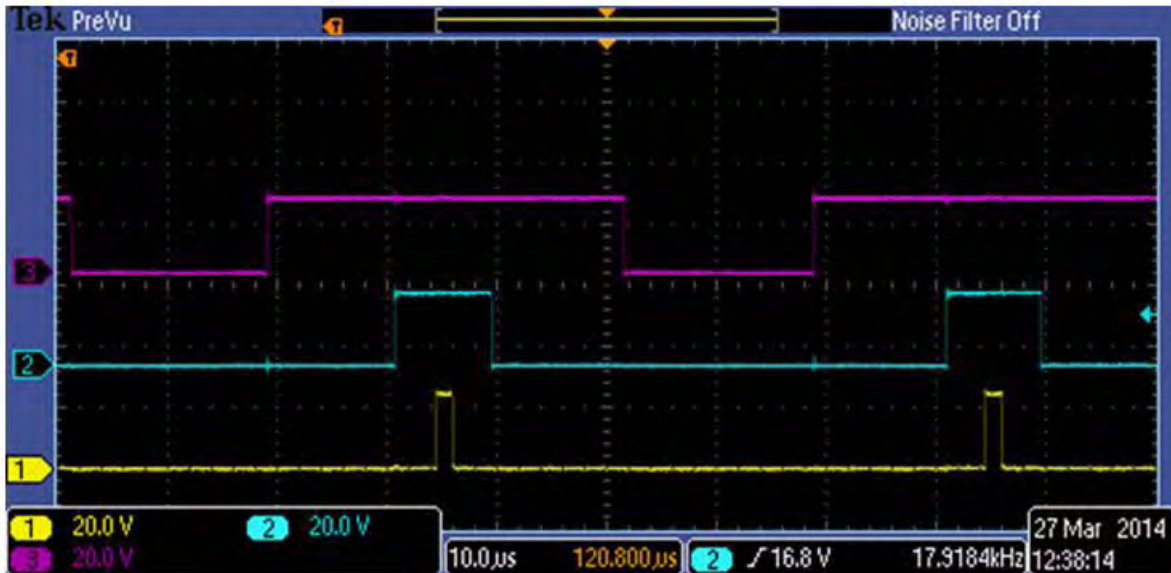
Figure 18. Alternate-Reverse PWM Switching Pattern
