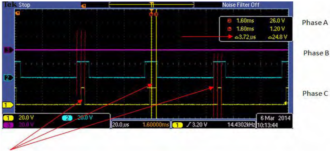
Figure 4. Low-Speed ADC Measurement Timing
