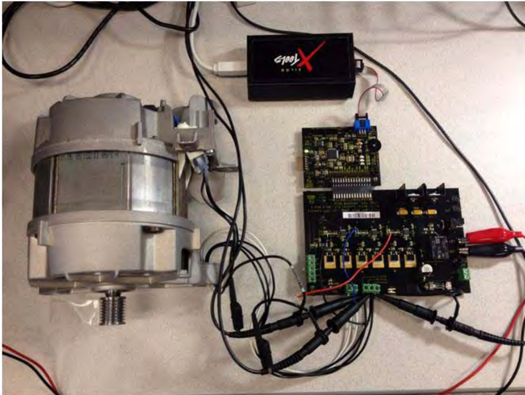
Figure 21. The MultiMotor Development Kit with AC Inductor Motor
